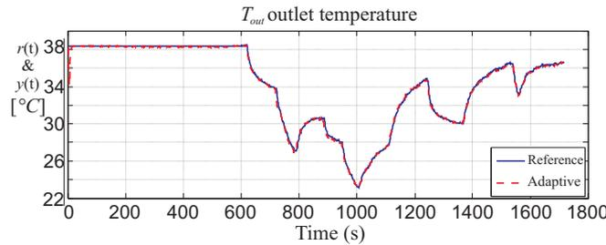
**Figure 9.** Outlet temperature controlled by the adaptive controller.
