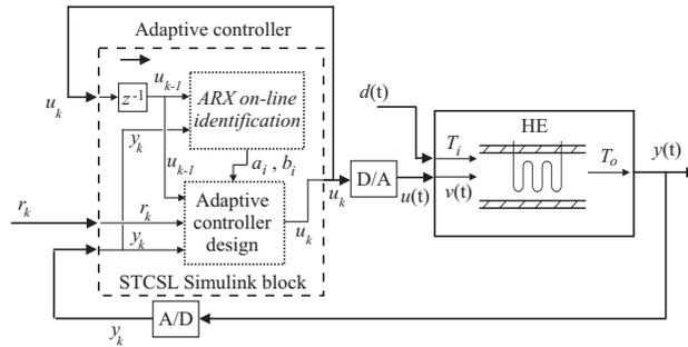
Figure 10. Block diagram of the HE system controlled by the adaptive regulator.
