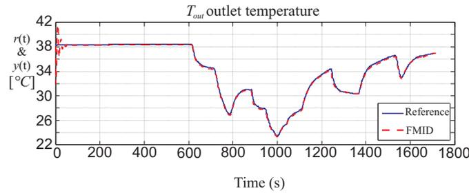
**Figure 8.** Outlet temperature controlled by the fuzzy controller estimated by the FMID tool.
