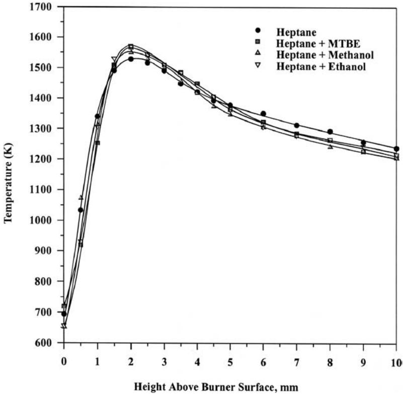
Figure 2. Flame temperatures.
