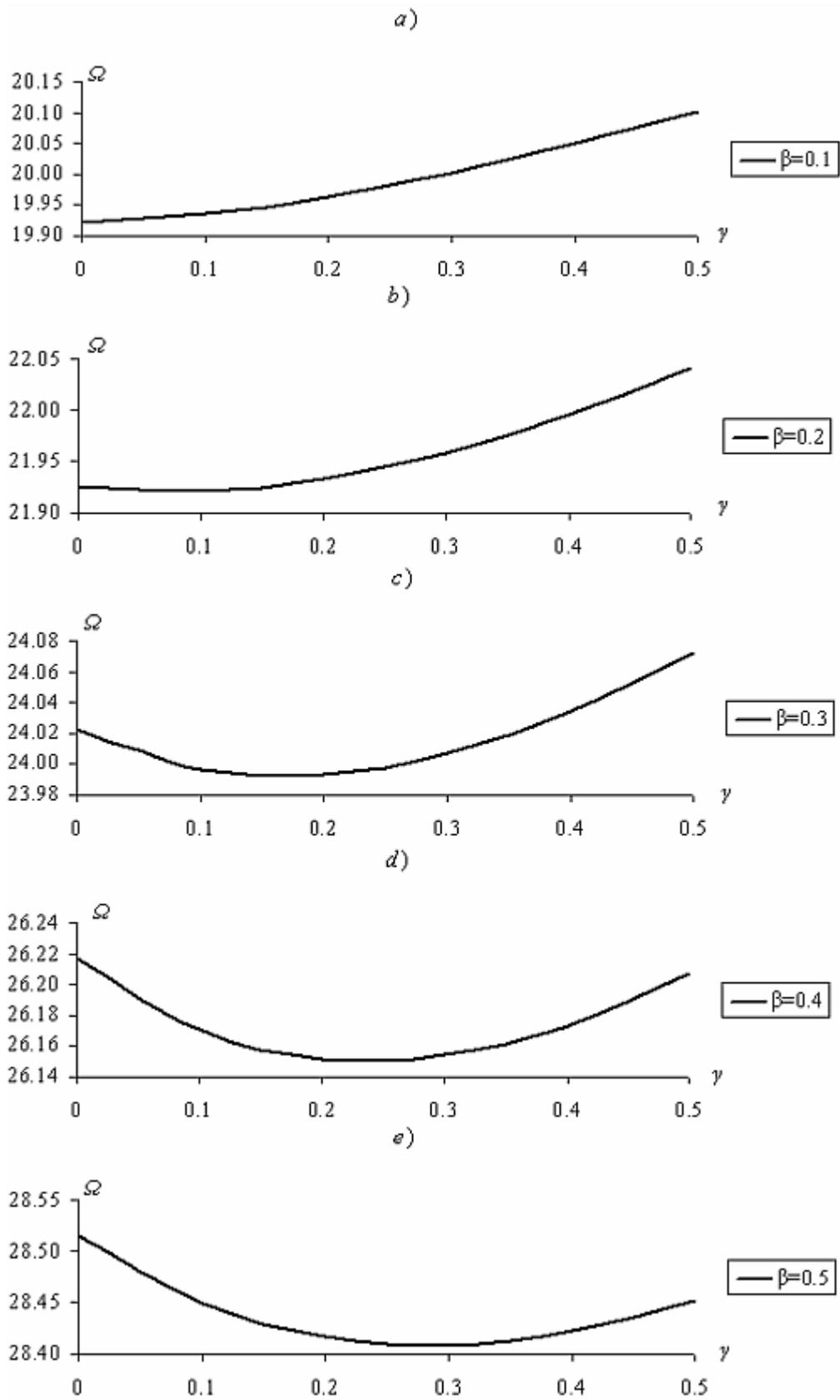
Figure 3.7. Dimensionless first natural frequency for a fixed-fixed curved beam of  $\lambda_0=\pi$  and  $\delta=0.1$  vs.  $\gamma$ -width variation parameter for different  $\beta$  values ( $n=100$ )
