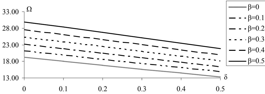
Figure 3.9. Dimensionless first natural frequency for a fixed-fixed curved beam of  $\lambda_0=\pi$ ,  $\gamma=0.1$  vs.  $\delta$ -linear curvature variation parameter for different  $\beta$  values ( $n=100$ )
