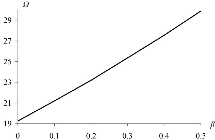
Figure 3.6. Dimensionless first natural frequency for a fixed-fixed curved beam of  $\lambda=\pi$  and  $\gamma=0.1$  vs.  $\beta$ -linear cross-section variation parameter ( $n=100$ )
