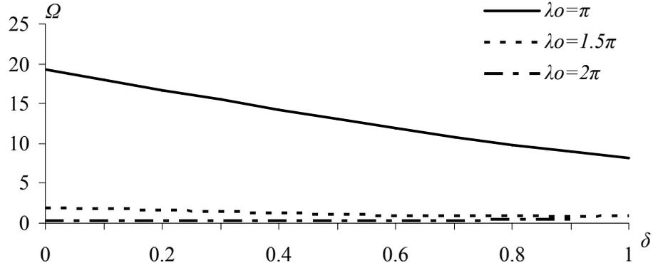
Figure 3.2. Dimensionless first natural frequency for a fixed-fixed curved beam of different  $\lambda_0$ 's vs.  $\delta$ -linear variation parameter ( $n=100$ )
