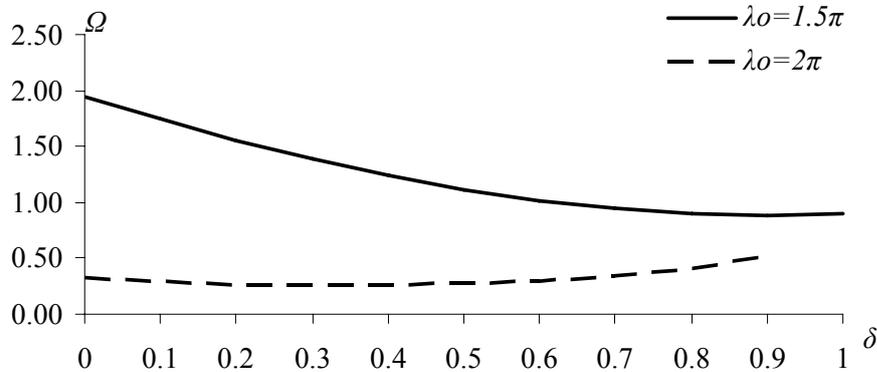
Figure 3.3. Dimensionless first natural frequency for a fixed-fixed curved beam of two different  $\lambda_0$ 's vs.  $\delta$ -linear variation parameter ( $n=100$ )
