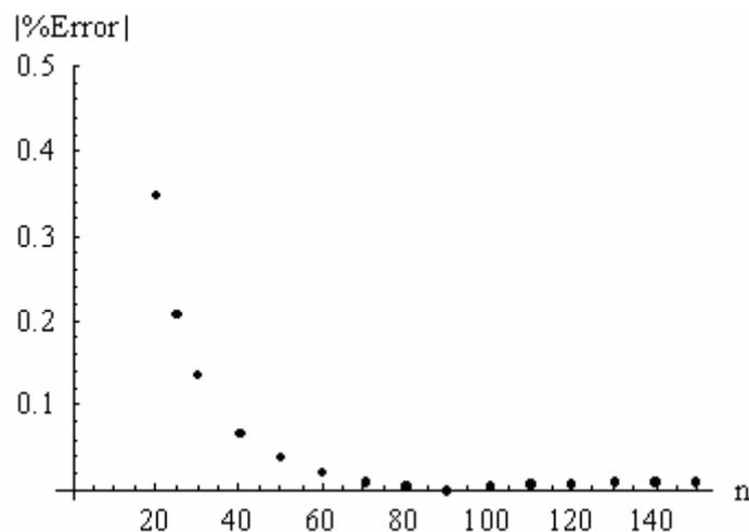
Figure 3.1. Absolute percentage error of dimensionless first natural frequency  $\Omega$  for a fixed-fixed curved beam of  $\lambda=\pi$  vs. n-number of grids
