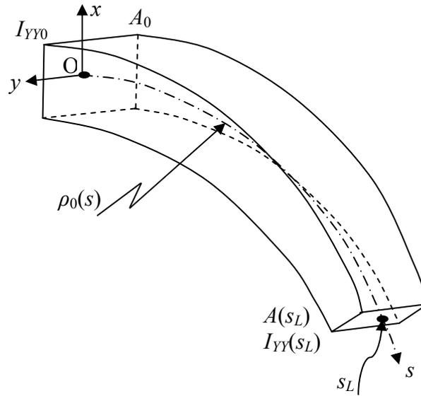
Figure 2.1. A representative curved beam with variable curvature and cross section
