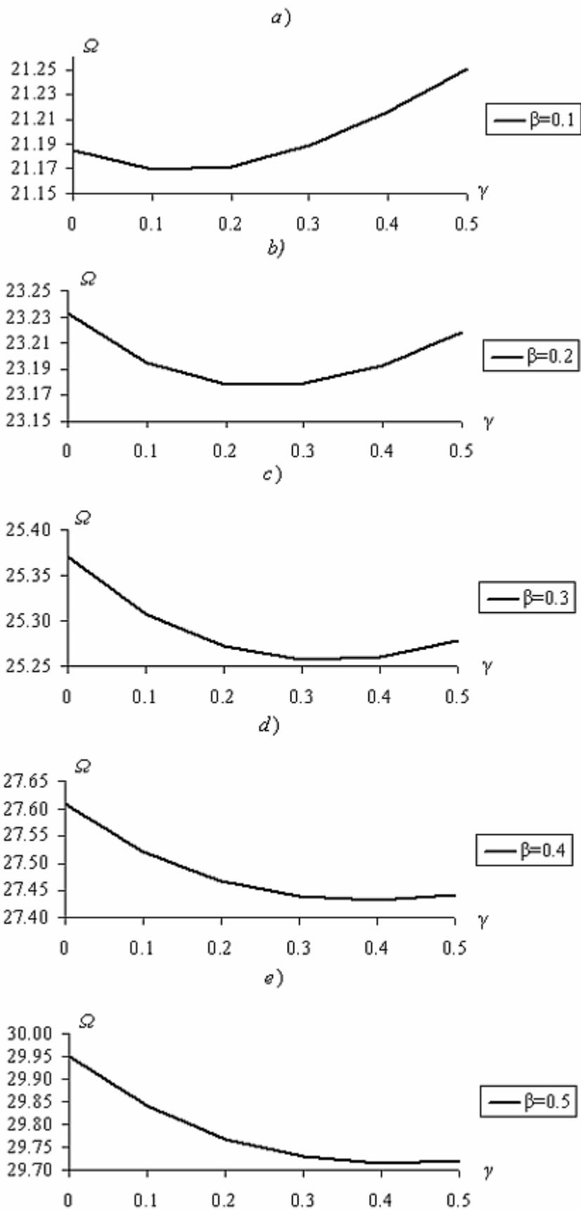
Figure 3.5. Dimensionless first natural frequency for a fixed-fixed curved beam of  $\lambda=\pi$  vs.  $\gamma$ -width variation parameter for different  $\beta$  values ( $n=100$ )
