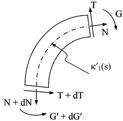
Figure 2.2. A differential curved beam with internal forces and bending moment
