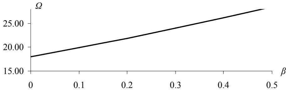
Figure 3.8. Dimensionless first natural frequency for a fixed-fixed curved beam of  $\lambda_0=\pi$ ,  $\delta=0.1$  and,  $\gamma=0.1$  vs.  $\beta$ -linear depth variation parameter ( $n=100$ )
