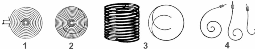
Figure 1.1. Balance springs: (1) flat spiral, (2) Breguet overcoil, (3) chronometer helix, showing curving ends, (4) early balance springs.
