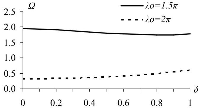
Figure 3.4. Dimensionless first natural frequency for a fixed-fixed curved beam of two different  $\lambda_0$ 's vs.  $\delta$ -quadratic variation parameter ( $n=100$ )
