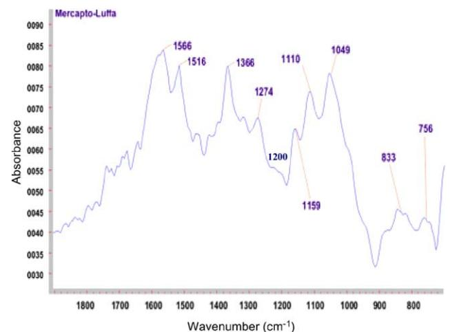
Fig. 7. FTIR-ATR spectra of mercapto modified luffa fiber.
