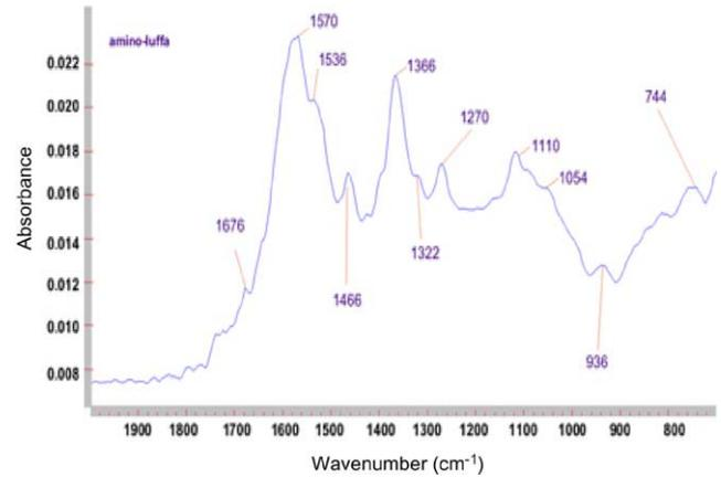
Fig. 6. FTIR-ATR spectra of amino modified luffa fiber.
