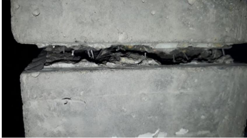
Figure 4.2. SF45/35\_3D\_075-1 specimen after cracking
