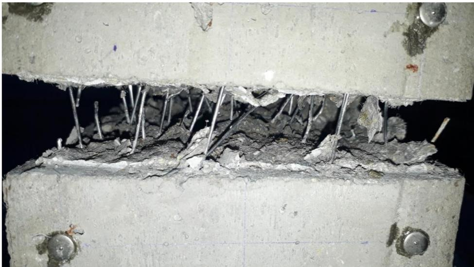
Figure 4.14. SF65/60\_3D\_075+PVA-3 specimen after cracking
