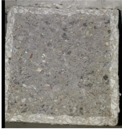
Figure 4.29. PVA group specimen after cracking
