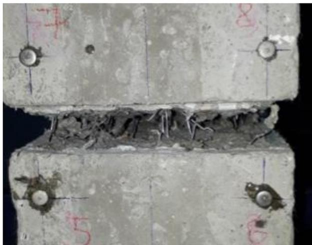
Figure 4.8. SF45/35\_3D\_075+PVA-3 specimen after cracking
