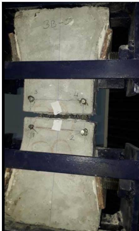
Figure 4.20. SF65/60\_5D\_075+PVA-3 after cracking
