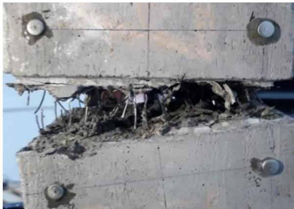
Figure 4.7. SF45/35\_3D\_075+PVA-2 specimen after cracking
