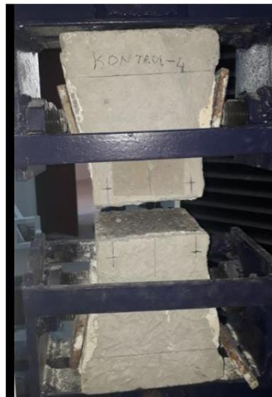
Figure 4.31. Normal concrete group specimen after cracking
