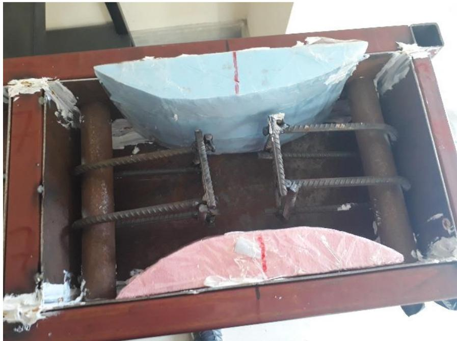
(f) T6 (steel bars with short bars welded at the ends, free distance: 60 mm)
