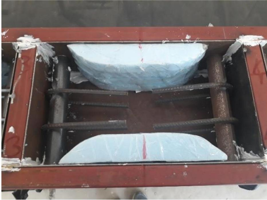
(c) T3 (straight steel bars, free distance: 45 mm)
