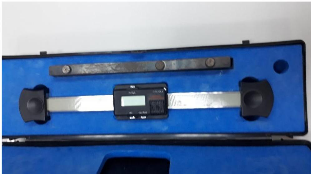
Figure 3.22. Digital movement gauge
