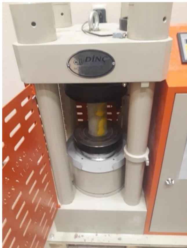
Figure 3.27. Digital compressive test machine
