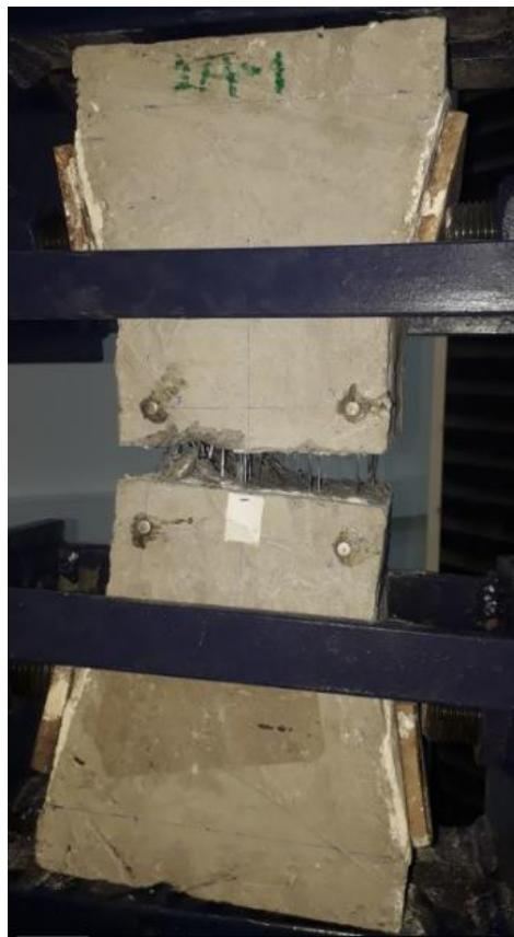
Figure 4.10. SF65/60\_3D\_075-1 specimen after cracking
