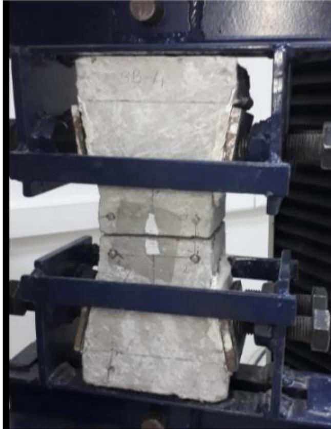
Figure 4.19. SF65/60\_5D\_075+PVA-2 specimen after cracking
