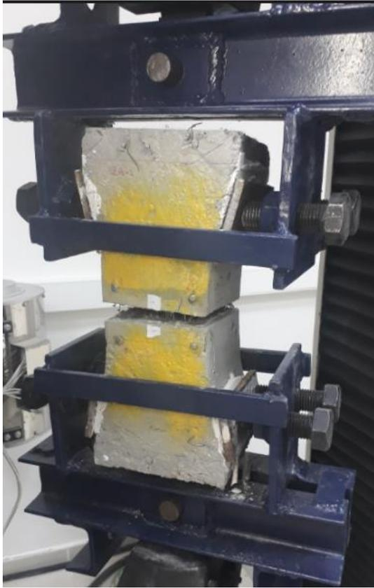
Figure 4.13. SF65/60\_3D\_075+PVA-2 specimen after cracking
