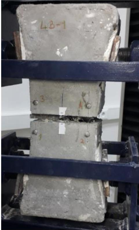
Figure 4.25. SF65/60\_3D\_125+PVA-1 specimen after cracking
