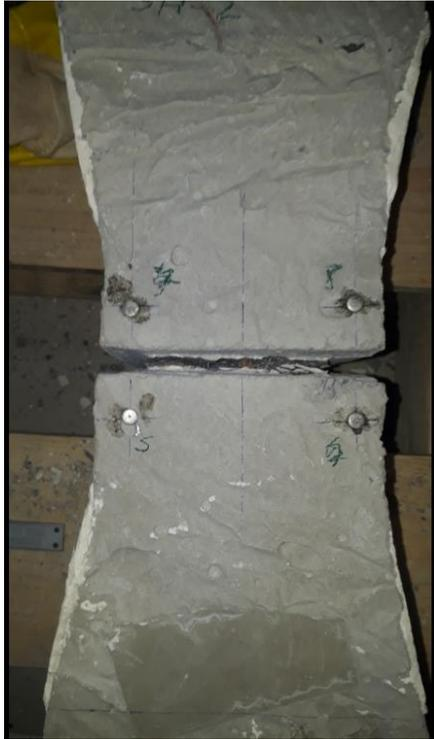
Figure 4.17. SF65/60\_5D\_075-2 specimen after cracking
