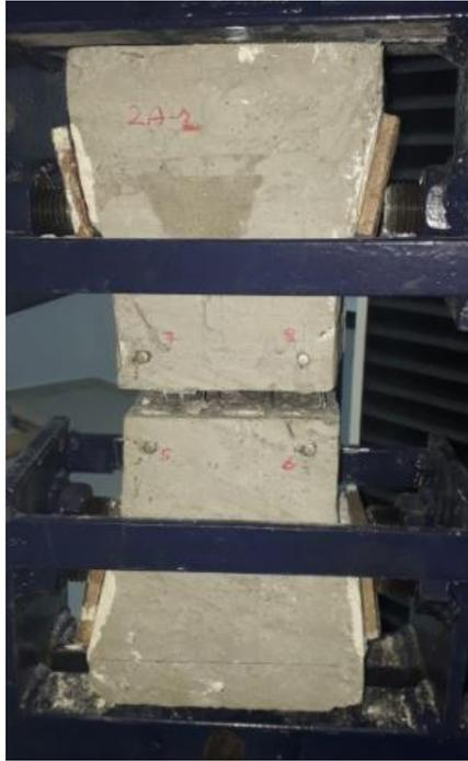
Figure 4.11. SF65/60\_3D\_075-2 specimen after cracking
