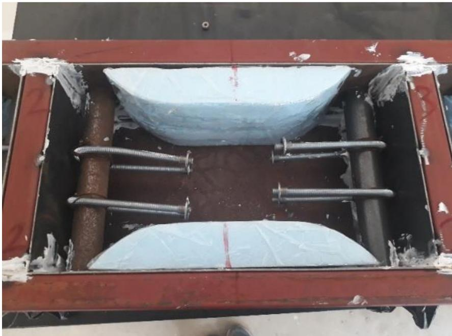
(b) T2 (Cold-formed threaded rods with flange nuts, free distance: 80 mm)
