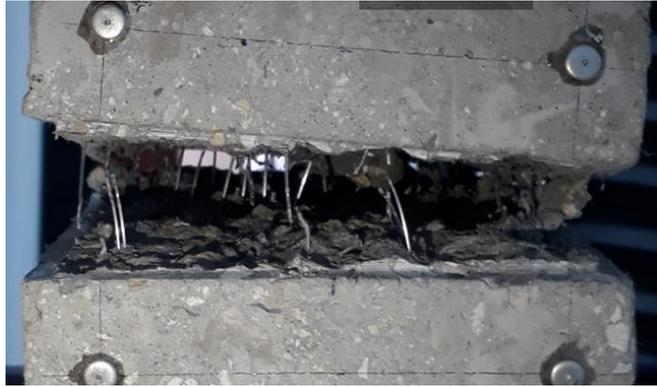
Figure 4.6. SF45/35\_3D\_075+PVA-1 specimen after cracking
