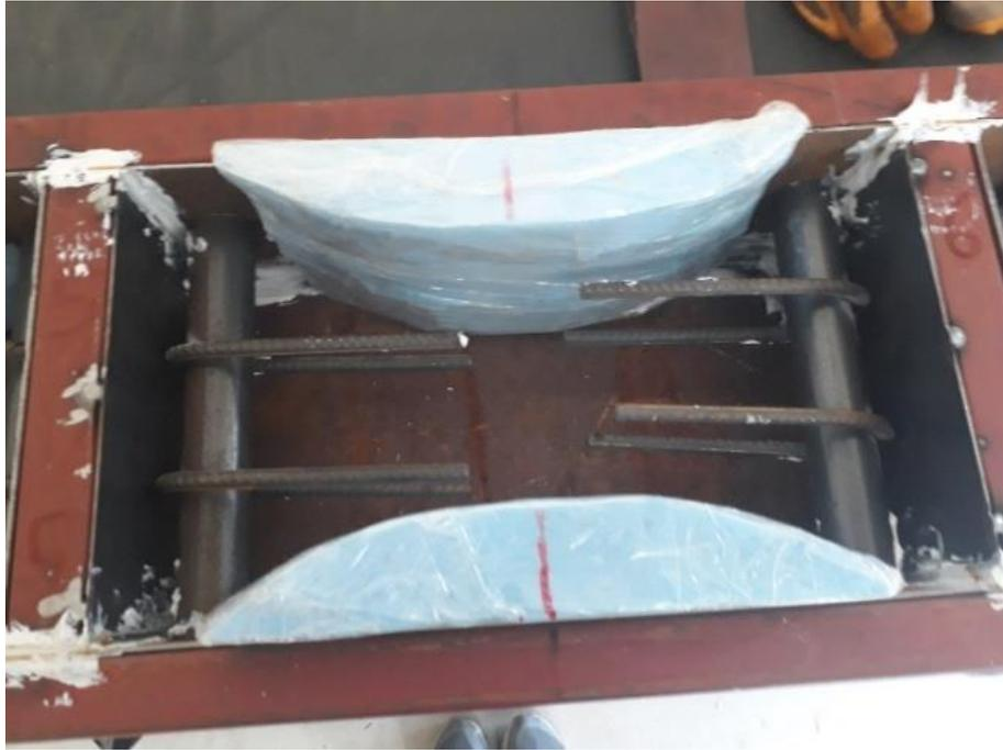
(e) T5 (straight steel bars, free distance: 60 mm)
