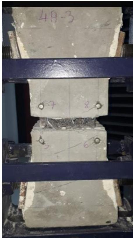
Figure 4.22. SF65/60\_3D\_125-1 specimen after cracking
