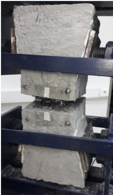
Figure 4.26. SF65/60\_3D\_125+PVA-2 specimen after cracking
