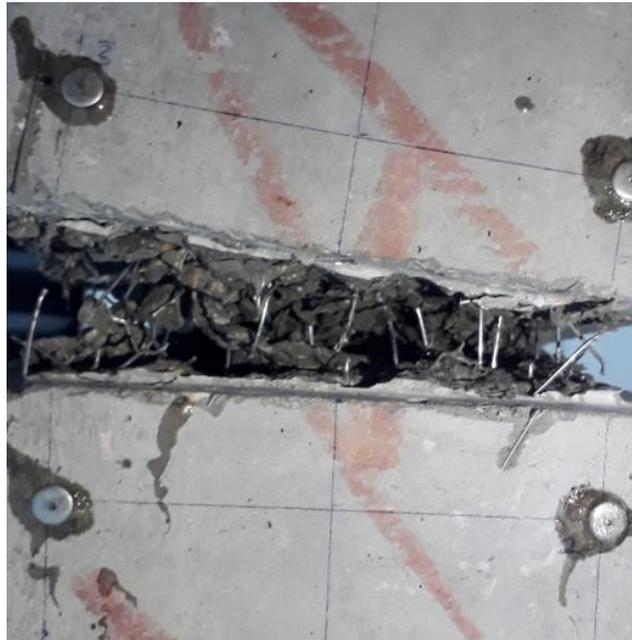
Figure 4.3. SF45/35\_3D\_075-2 specimen after cracking
