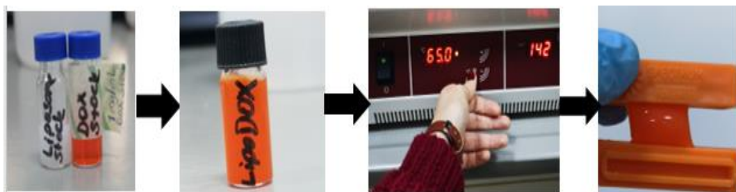
Figure 3.7. Incubation step for DOX loading step into liposomes
