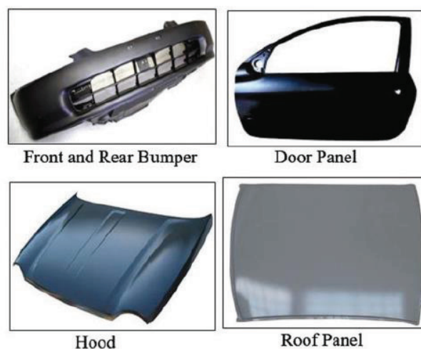
Figure 2.5. The parts manufactured by using carbon-glass fiber reinforced epoxy hybrid composites (Source: Ravishankar, Nayak, and Kader 2019)
