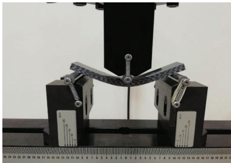
Figure 4.7. An angle-ply sample under bending test
