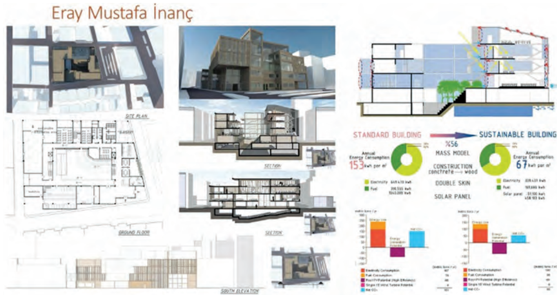
FIGURE 1. The successful student's project incorporated the use of natural light, natural ventilation, sustainable materials (totally constructed out of wood), double skin façade, shading elements, green elements, rain water collection, reuse of gray water, and solar panels. The proposed design had achieved a 56% reduction in annual energy consumption.
