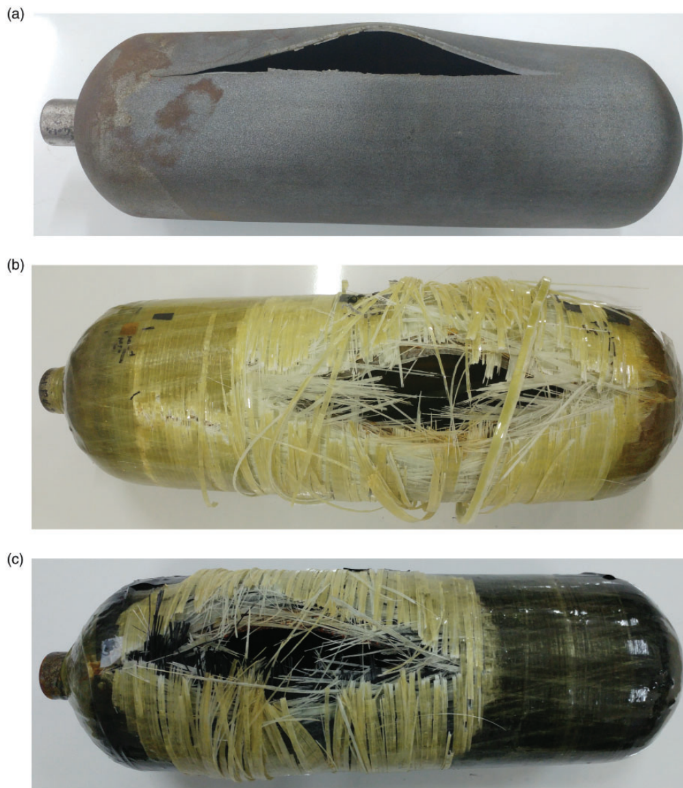
Figure 8. (a) Steel liner, (b) glass fiber COPVs, (c) hybrid fiber COPVs after burst pressure testing.
