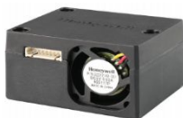
Fig. 5. Particle sensor used in air quality sensor pack
