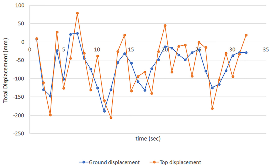
Fig. 17. Time–displacement data at the ground and top for Portion A.
