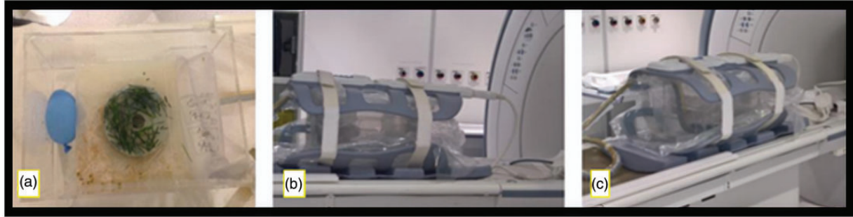
Fig. 6. (a) Experiment set-up showing the phantom which includes vein mimicking sapphire structure on the left image inside the custom-made phantom holder, including a water balloon and air bag, which is connected to the air ventilator to push the phantom to simulate the breathing motion. (b, c) Images of the 8 Channel Torso Coils including the CBS transducer inside the assemble for sonication side and orthogonal views, respectively (© IMSaT, Dundee, Scotland, UK).
