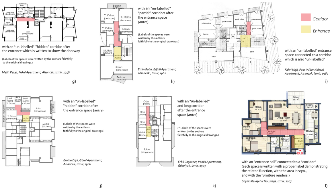
Figure 3. Plan examples having a corridor—whether labelled or unlabelled—to provide transition between the rooms. Sources: g,h. Güner 2005; i. Nişli 1961; j,k. Archives of Izmir Metropolitan and Konak Municipalities; l. Soyak 2009.
