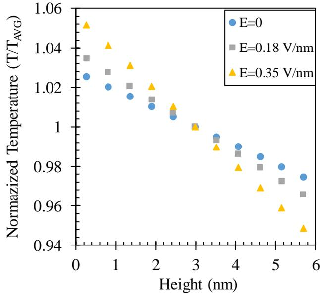
Fig. 2: Normalized temperature profiles of water molecules under varying electric field strengths.
