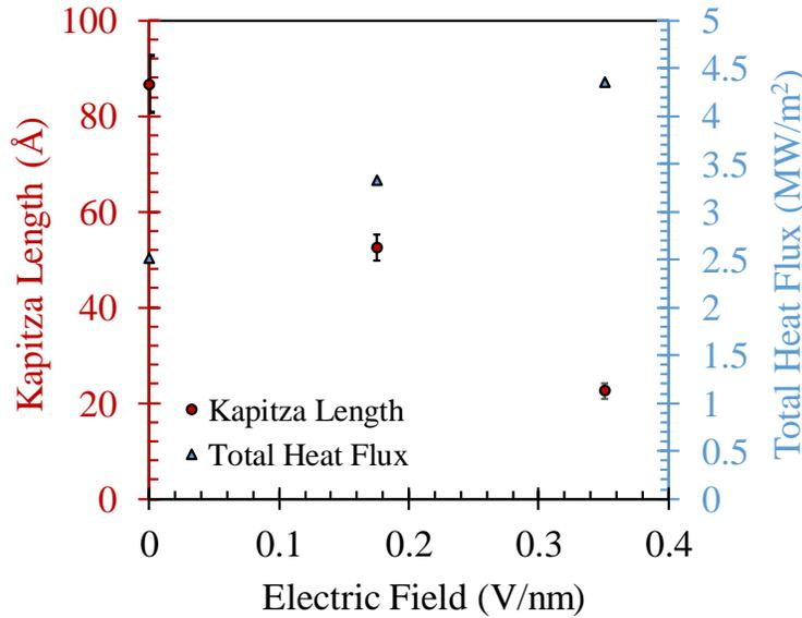
Fig. 4: Kapitza length and total heat flux variation with electric field strength.
