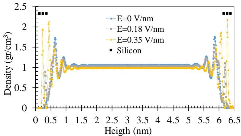
Fig. 3: Density profiles of water molecules under varying electric field strengths.
