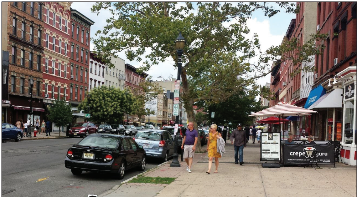
Figure 6.3. Creating a buffer between pedestrians and moving vehicles by the use of landscape and street furniture. (Source: Schmitt, 2016)
