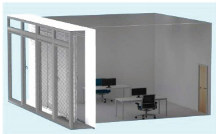
Figure 3.12. 3D view of Relux Model showing Double Skin Facade
