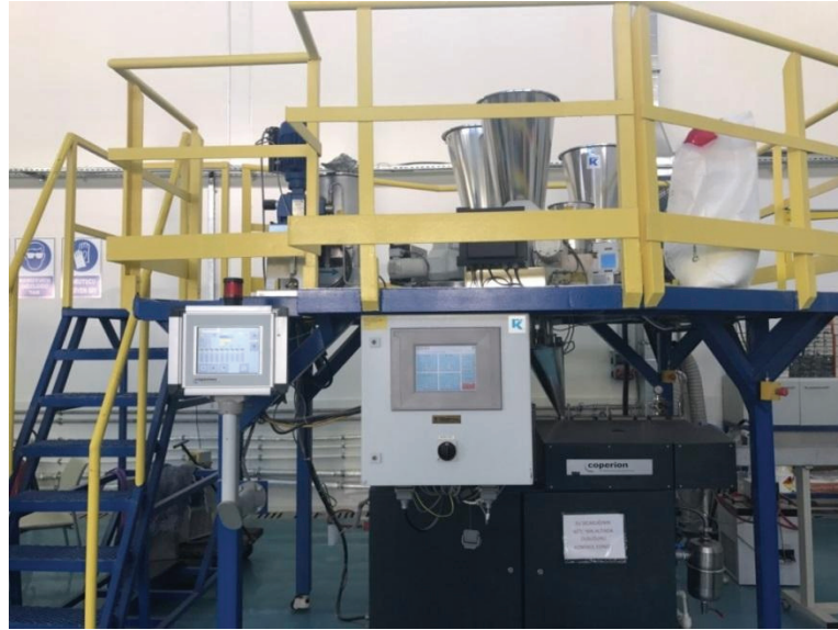
Figure 3.1 Sample blends were processed in the double screw Coperion ZSK-18 brand extruder.
