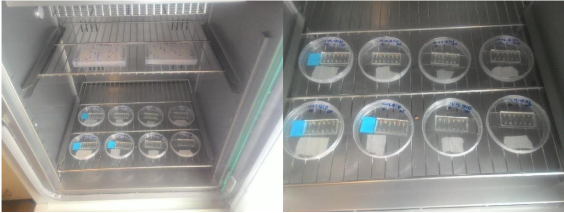
Figure 2.4. View of the growth chamber (left) and the working of the chips (right).
