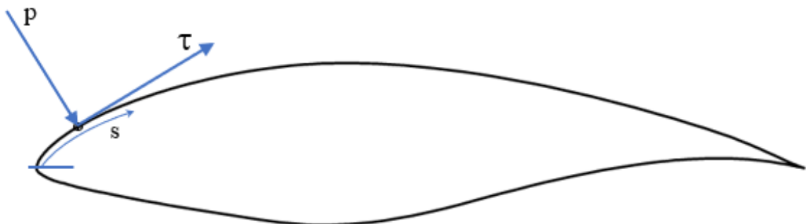
Figure 14. Stress distributions on an airfoil
