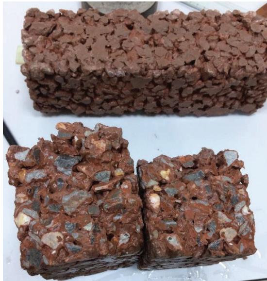
Figure 4.15 The beam sample after the flexural strength test
