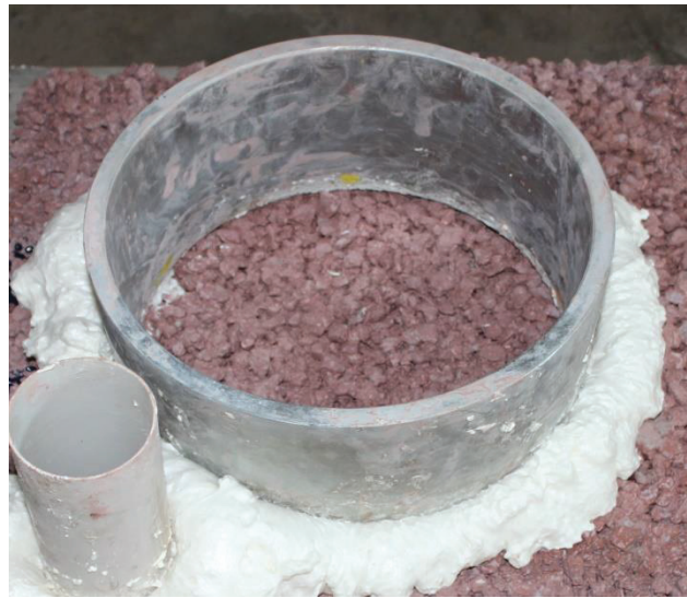
Figure 3.16 Insulation ring with aerogel to measure permeability rate
