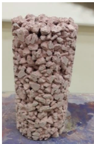
Figure 3.13 Sample to measure the hardened density of pervious concrete
