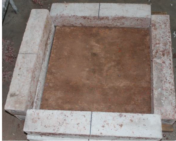
Figure 3.15 The mold for pervious pavement
