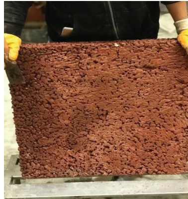
Figure 4.11 The clogging of the pervious concrete due to the excess paste
