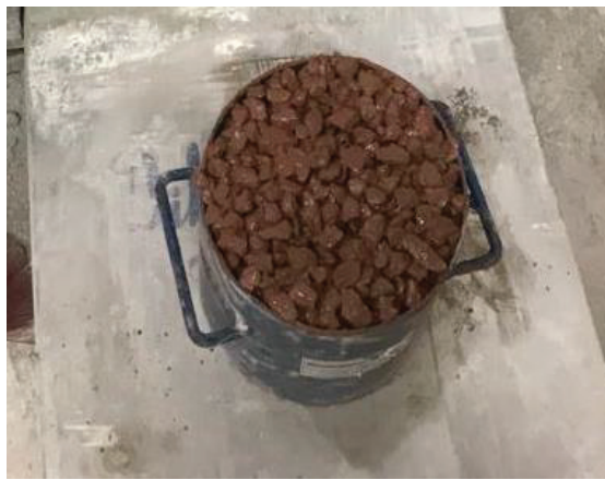
Figure 3.12 Density of freshly mixed pervious concrete
