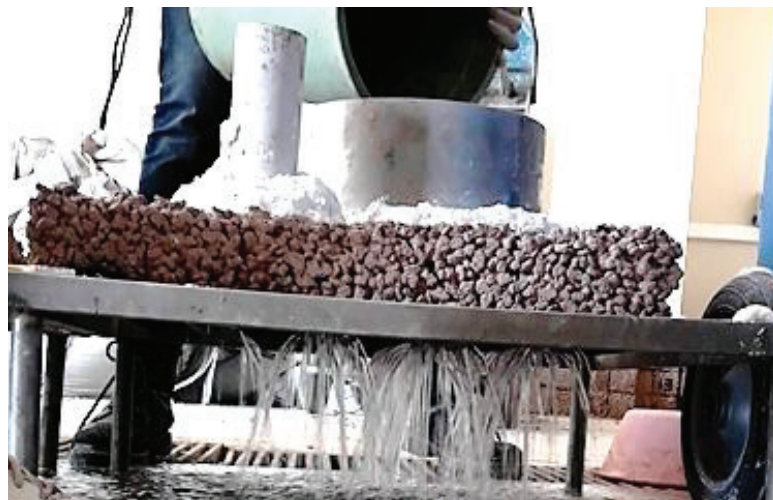
Figure 3.17 The mechanism to measure the permeability of pervious pavement
