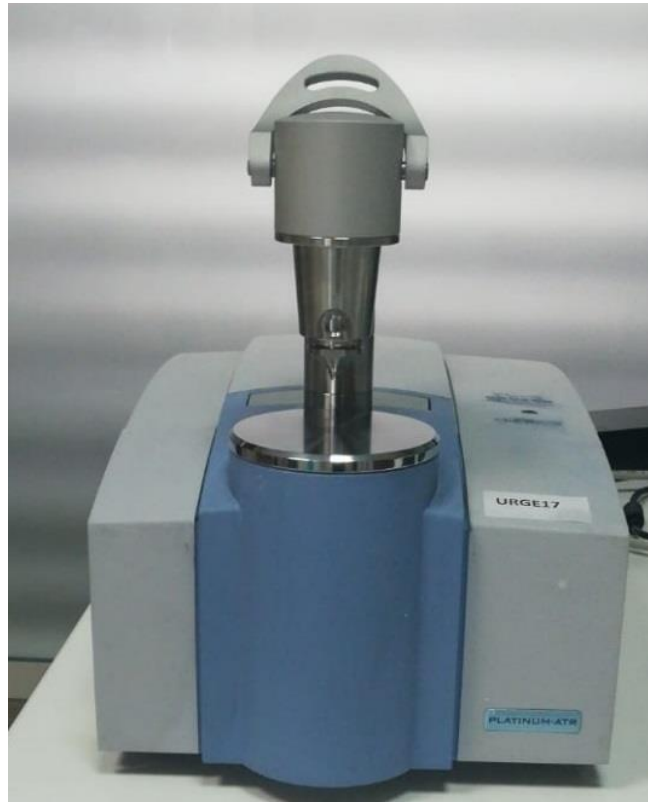
Figure 2.3. Fourier transform infrared spectroscopy with ATR instrument.
