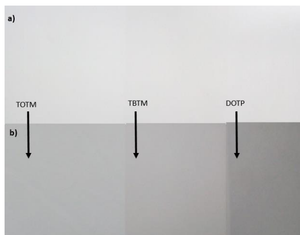
Figure 3.16. Color changes of artificial leathers obtained by using TOTM, TBTM, DOTP after 70 °C heat treatment a) initial b) after 24 hours
