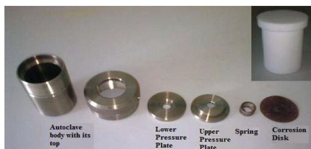
Figure 3.1. Steel autoclave and Teflon vessel. (Source: Onen, 2011).
