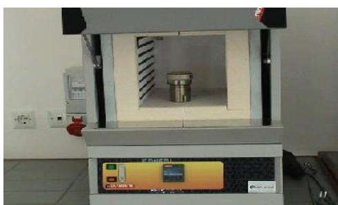
Figure 3.2. Steel autoclave placed in oven. (Source: Onen, 2011).
