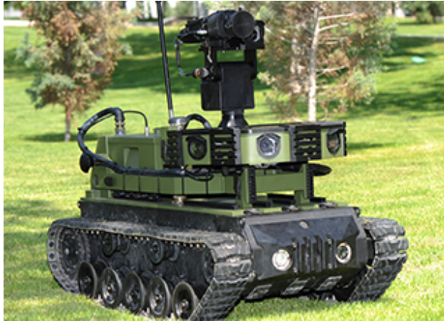
Figure 1.5. Aselsan's Kaplan, unmanned ground vehicle. (Source: Aselsan)
