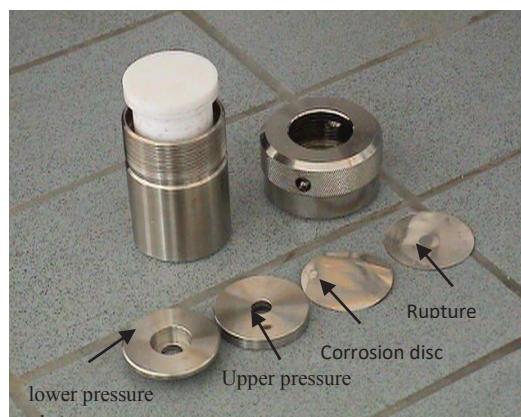
Figure 2.1. Parts and schematic representation of a stainless-steel autoclave. (Source: Şahin 9 )
