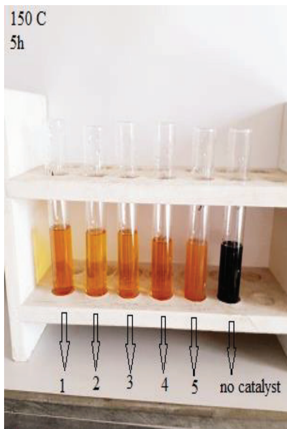
Figure 4.2. Lugol's test of the reactions with five different crystals and without any catalyst.
