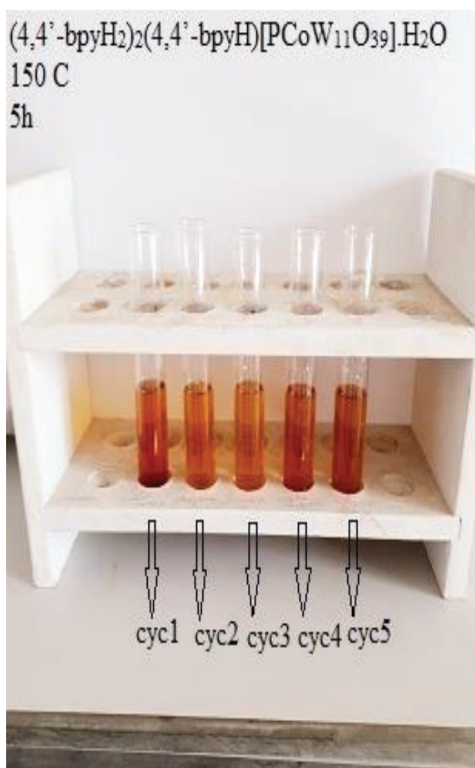
Figure 4.8. Lugol's test of the reaction with (4,4'-bpyH 2 ) 2 (4,4'-bpyH)[PCoW 11 O 39 ].H 2 O crystal for five cycles.
