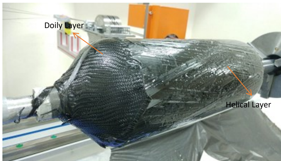
Figure 5.10. Doily and Helical Layers of COPVs.
