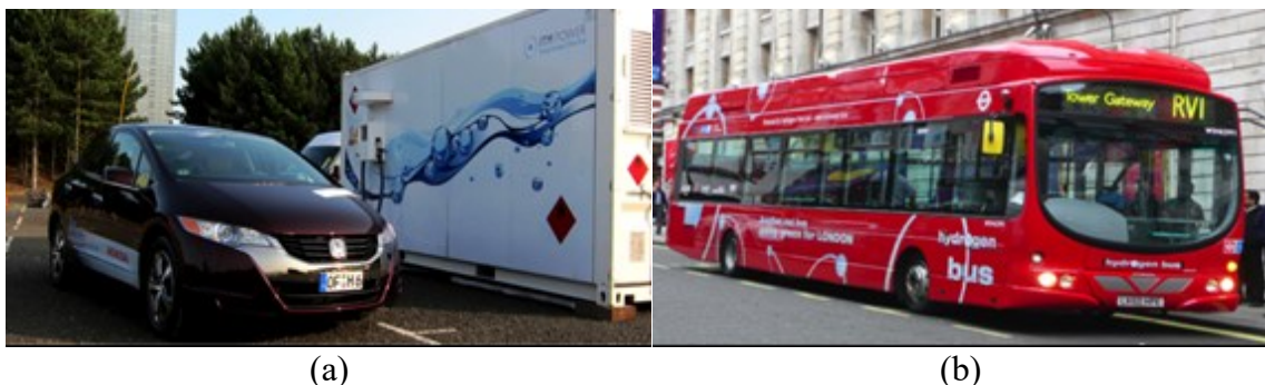
Figure 1.1. Onboard applications for hydrogen energy. (a) A hydrogen-powered fuel cell vehicle beside a hydrogen station, (b) a hydrogen-powered public transportation vehicle in London. (Source: Oyakhire, 2012)
