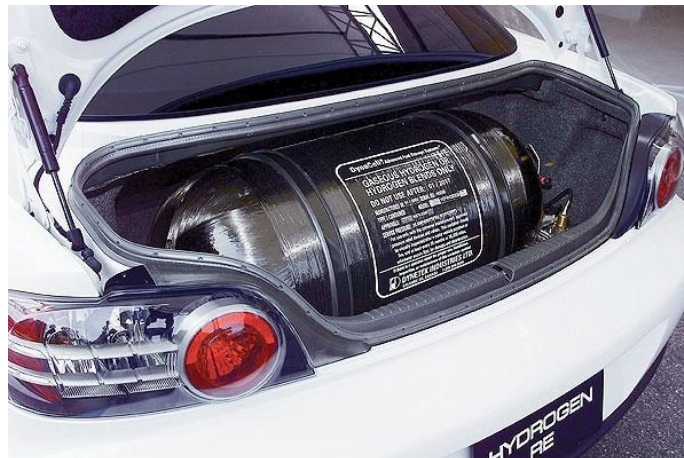
Figure 4.2. Composite overwrapped pressure vessel placement on a commercial vehicle.
