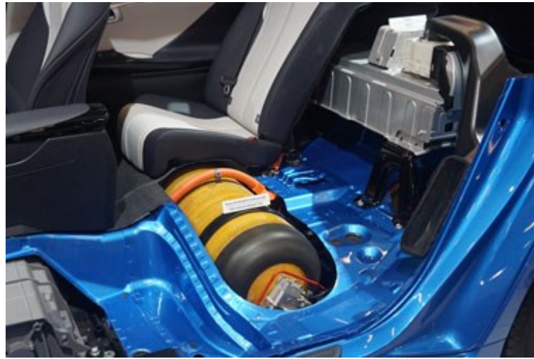
Figure 1.6. Typical positioning of a COPV on a commercial hydrogen-powered vehicle, Toyota Mirai. (Source: Lawrence Livermore National Laboratory, 2019)
