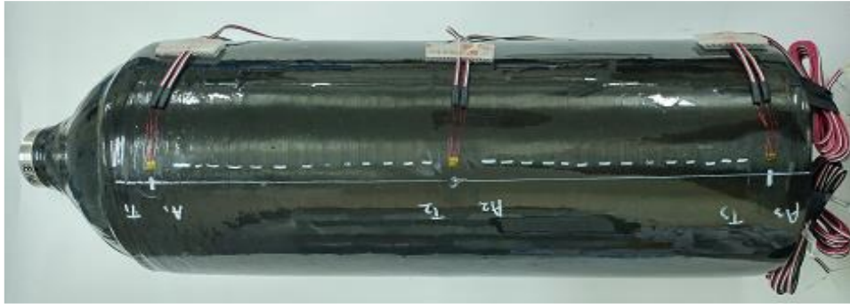
Figure 5.15. A photograph of the hydrostatic test specimen of Al-based carbon reinforced COPV before testing
