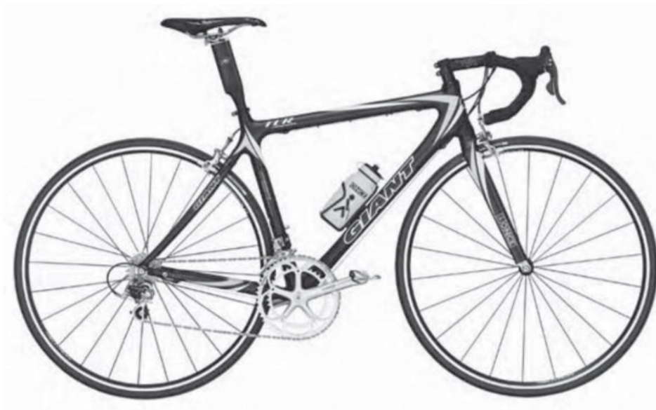
Figure 2.4. Lightweight race bicycle made of composite parts. (Source: Long, 2005)
