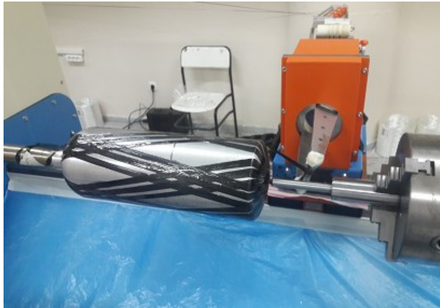
Figure 5.9. The helical winding of aluminum-based COPVs with the filament winding machine.
