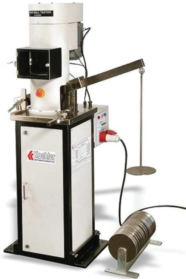
Figure 23 Four Ball Tester (Source: Koehler Instrument). 41
