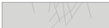
Fig. 14. A two dimensional vertical cross-section through a N–S striking profile of the faulted region around Varto caldera. The fault geometry is used as the model setup where each fault is assigned a different permeability. In all cases the top surface is unconstrained, whereas the x and lower y boundaries are fixed. The lower boundary of the model is assigned a starting temperature of 900 °C and the upper surface (free surface) is set at an atmospheric temperature of 25 °C.
