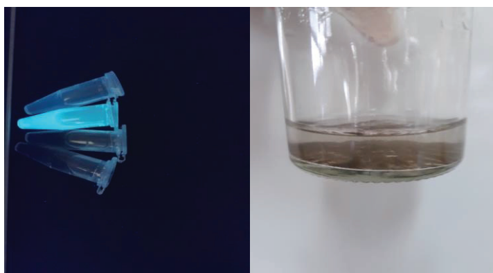
Figure 3.13 show the 5% Cu doped ZnSe after two days. luminescence property of nanocrystals disappeared and also brown precipitate occurred.
