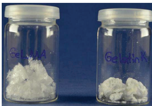
Figure 3.1 Images of GelMA and GelatinK polymers after lyophilization.
