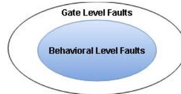
Figure 1. Relation of Gate and Behavioral Level Faults [1]
