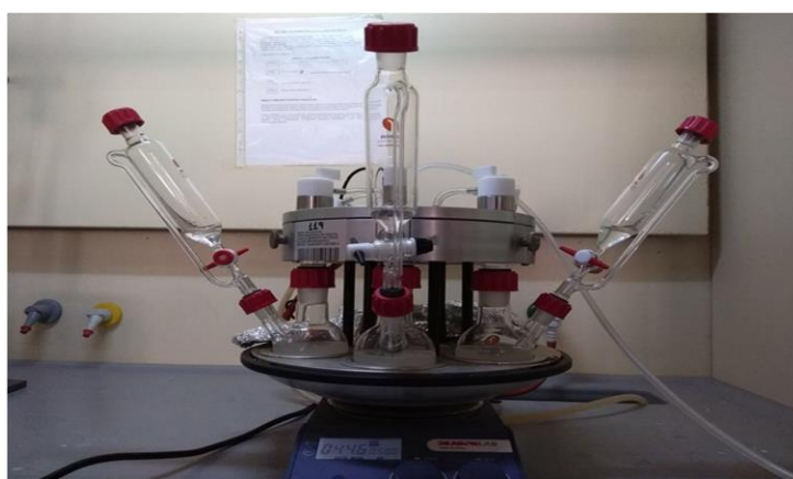
Figure 4.2. The reactor system for epoxidation of soybean oil
