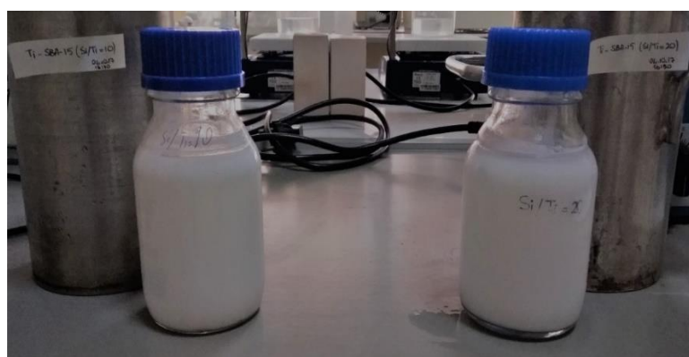
Figure 4.1. Ti-SBA-15 catalysts obtained hydrothermal synthesis in the autoclave.
