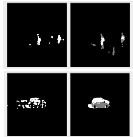
Fig. 5: The silhouettes at the left column are extracted by ABL, the ones at the right are extracted by MOG2 background subtraction algorithm [21].
