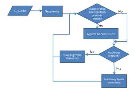
Figure 3. Flowchart of trajectory planning algorithm [Uzunoğlu et al., 2014].
