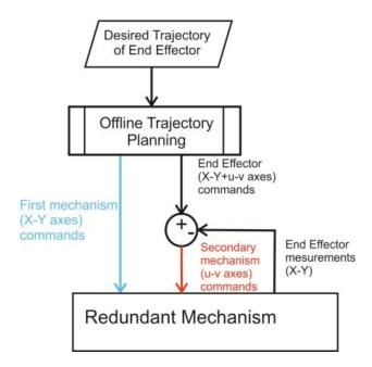
Figure 4. Control scheme of the proposed algorithm [Uzunoğlu et al., 2015].
