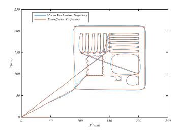
Figure 8. End-effector's and macro-mechanism's trajectories.
