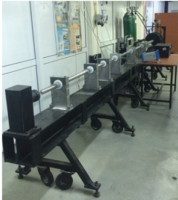
Figure 2.6. SHPB test setup in DTM Laboratory
