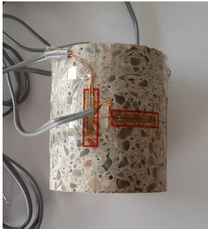
Figure 2.3. Strain Gage Glued Concrete Specimen
