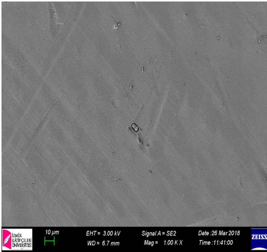
Figure 4.20. SEM image after E.coli filtration at T: 4°C and pH: 7.6.
