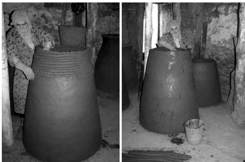
Figure 2.10. Woman adding up the clay coils (left) and polishing the almost-complete tandır oven (right) in Şık Village, Erzurum. (Source: Köşklü, 2005)
