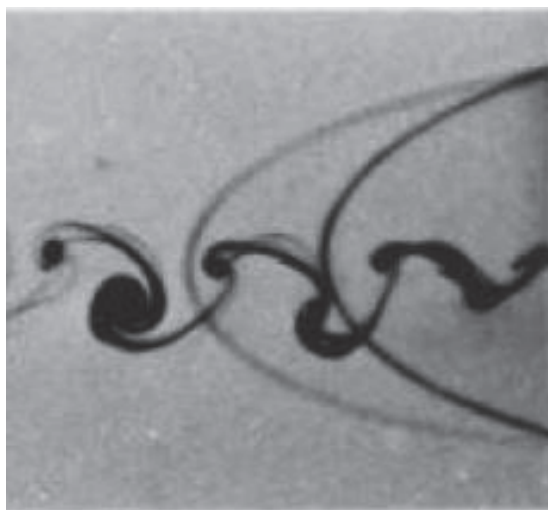
Figure 51. The visualization of the wake pattern of the NACA0012 in pitching motion by dye: \theta_m=0^\circ , \theta_a=4^\circ , l_{pa}=0.25 and k=8.96 at Re=1.2e4 . (Source: Koochesfahani (1989) )
