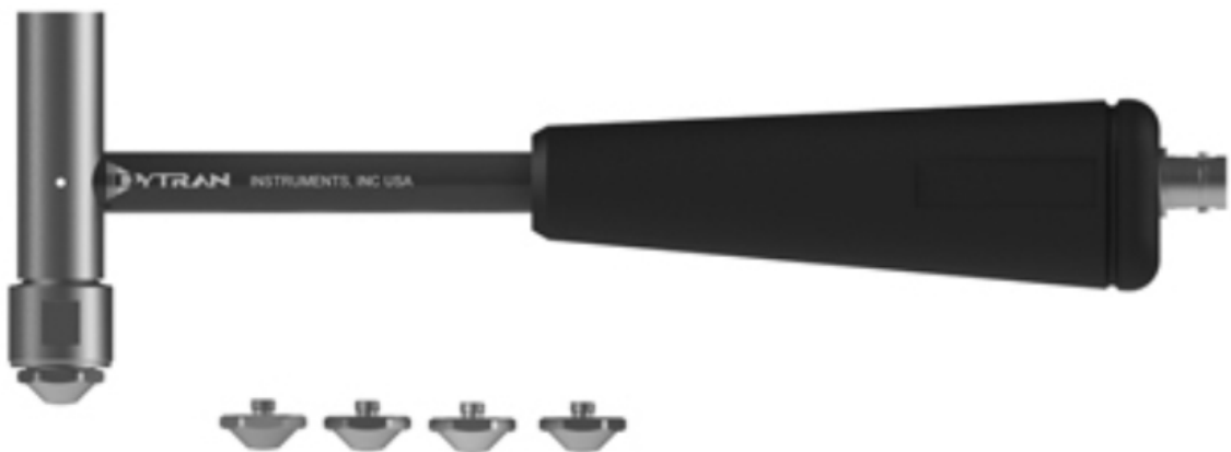
Figure 4.2. Impact hammer (Source: Dytran, 2018)
