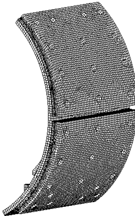
Figure 3.7. Finite element model of shoe
