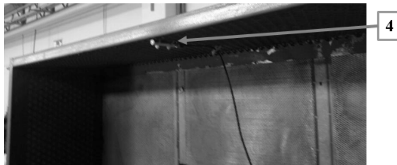
Figure 4.8. Installation of 2 nd microphone
