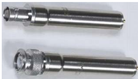
Figure 4.4. Microphone (Source: Norsonic, 2007)
