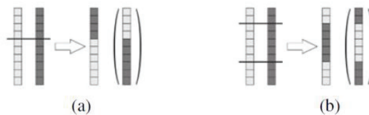
Figure 4.2. Types of crossover (a) One-point crossover (b) Two-point crossover (Source: Weise 2009)
