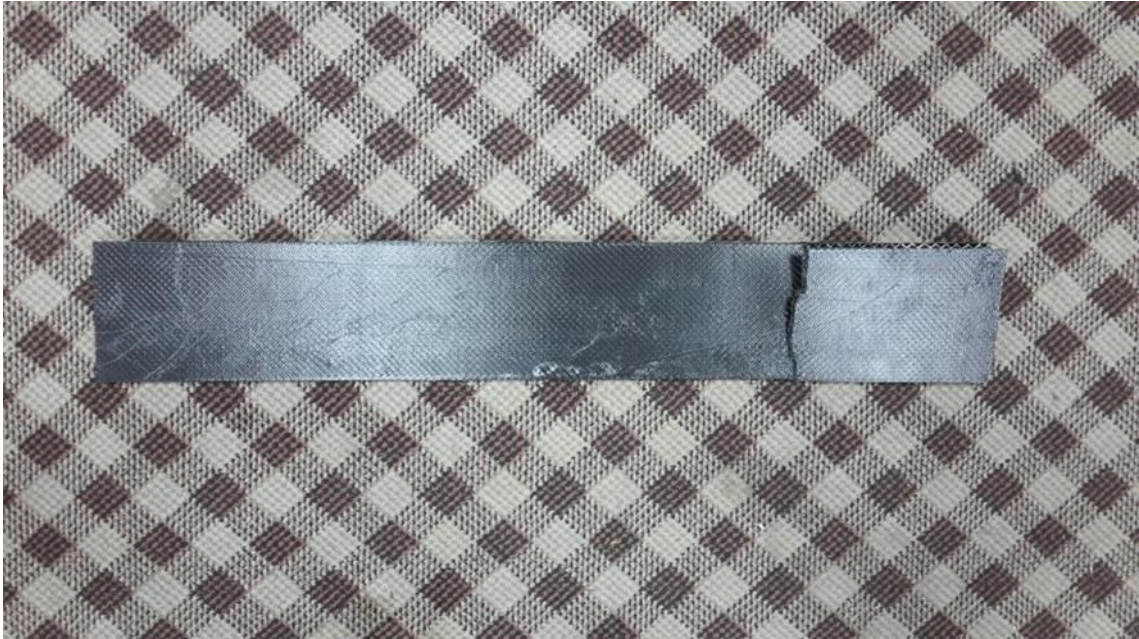
Figure 4.20 Sandwich beam face fracture
