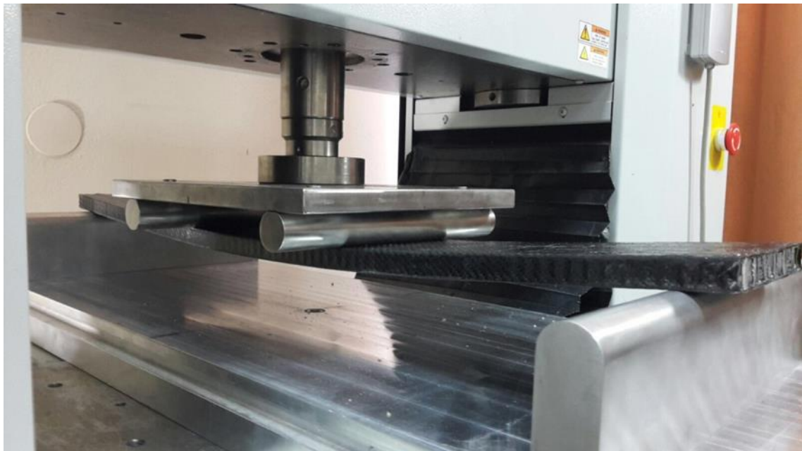
Figure 4.18 Four-point bending test
