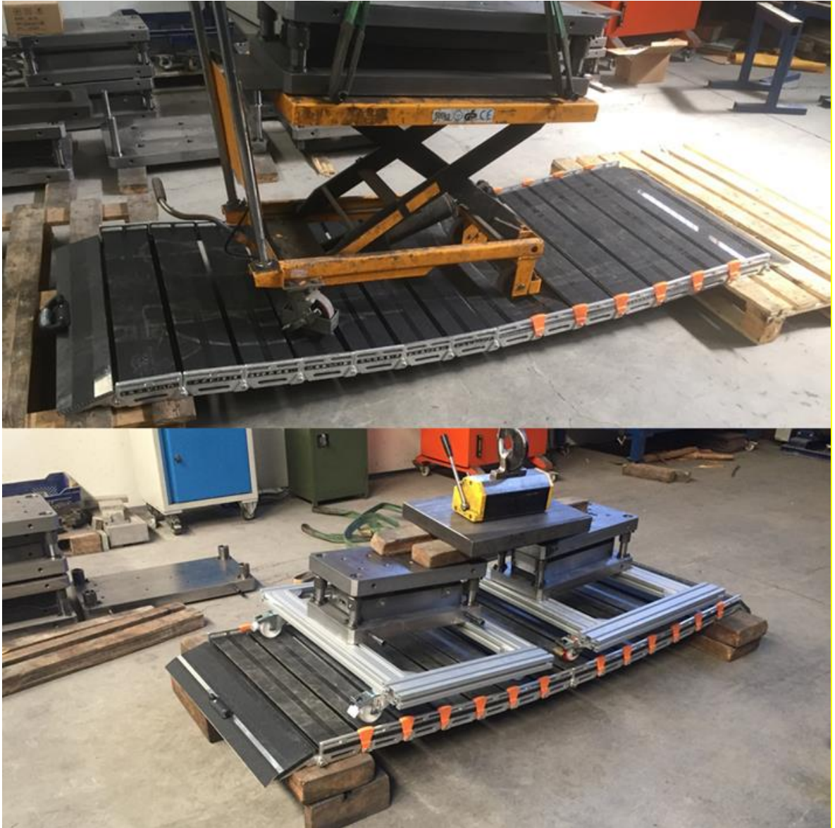
Figure 5.13 Field test under overload
