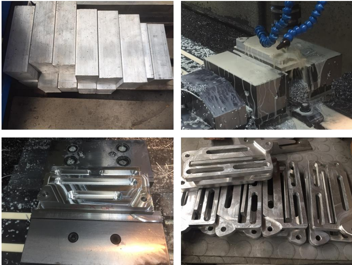
Figure 5.5 Link manufacturing with CNC milling machine
