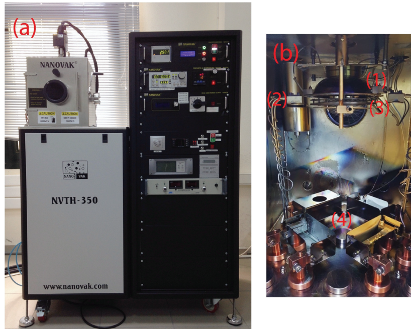
Figure 3.5. (a) The NVTH-350 Thermal Evaporation System in Quantum Device Laboratory. (b) (1) Radiative heater, (2) Quartz crystal monitor for precise thickness measurements, (3) sample holder, (4) Four boats (left-top: \text{SiO}_2 , right-top: Al, left-bottom: Cr, right-bottom: Au) are placed in the high vacuum chamber. The system allows to evaporate different materials without breaking the vacuum, which is essential for materials convenient to oxidation.
