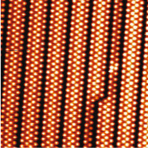
Fig. 1.1 15 \times 15 \text{ nm}^2 STM image recorded at 5 K ( V = \pm 0.05 \text{ V} , I = 200 \text{ nA} ) of the quasi perfect grating with a pitch of just 2 nm, formed by self-assembled symmetry breaking silicene nanoribbons, 1.6 nm in width. Adapted from Fig. 2 of Ronci et al. (2010)
