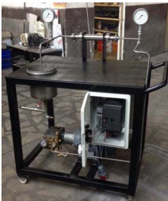
Figure 6.21. The filtration set-up used in MWCO and flux determinations.
