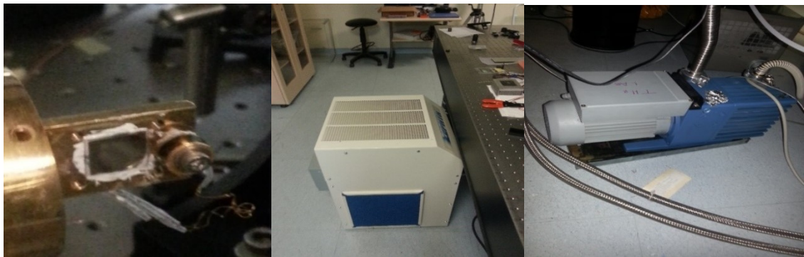
Figure 3.8. Sample holder, compressor and pump.
