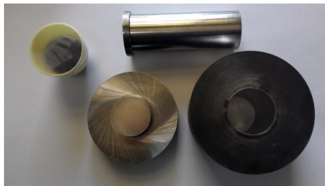
Figure 5.3. Calcined powder and tablet press mold in the alumina container.
