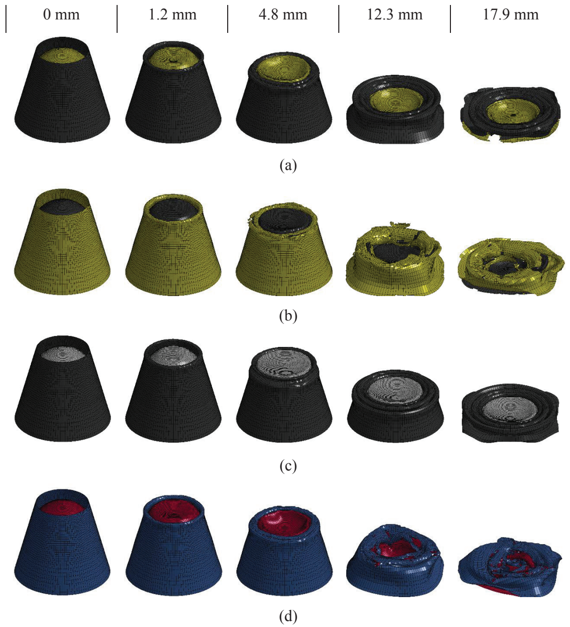
Figure 5.25. The deformation histories balanus placed in the center of sandwich structure (a) Heat-treated shell and as-received core (b) Heat-treated core and as-received shell (c) Heat-treated both of core and shell, and (d) As-received both of core and shell.
