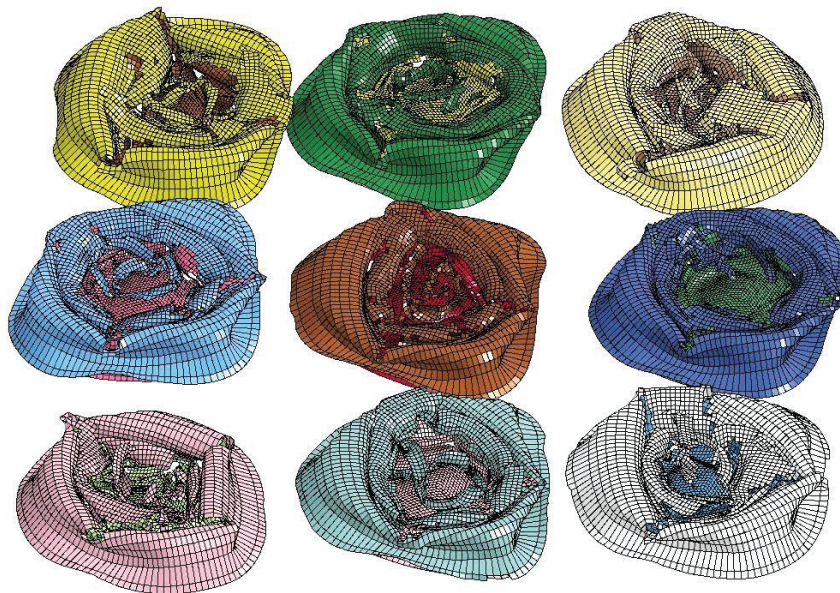
Figure 5.24. Deformed view of sandwich structures of (a) all front (b) all back (c) one-front / one-back, and (d) front-row / back-row.
