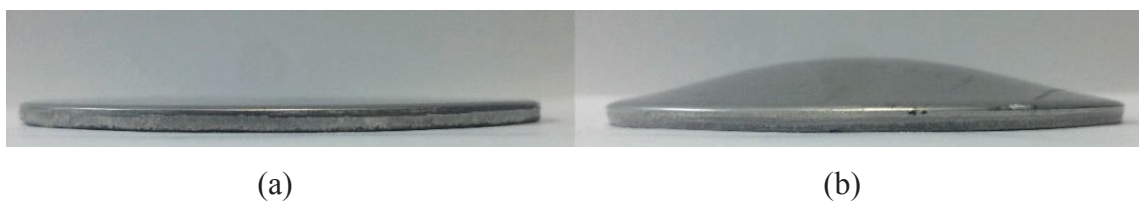
Figure 5.1. (a) Undeformed plate and deformed plates with impact velocities of (b) 32.75 m/s (c) 36.37 m/s, and (d) 39.78 m/s.
