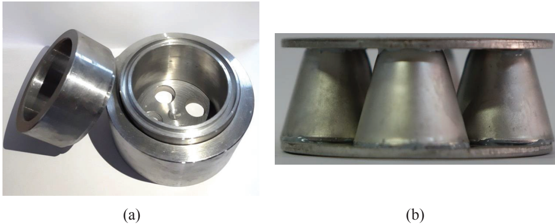
Figure 3.2. (a) Template for preparation sandwich specimens, and (b) A sample of balanus sandwich
