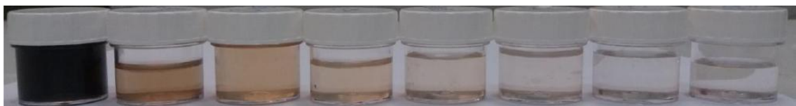
Figure 6.40. Color change of wastewater (without pre-treatment) (from left to right; original wastewater, UF-1 (disperal, P2), UF-2 (TTB), NF (one, two, three and four layers, respectively)).
