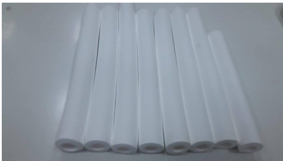
Figure 6.1. The extruded tubular \alpha -alumina supports.
