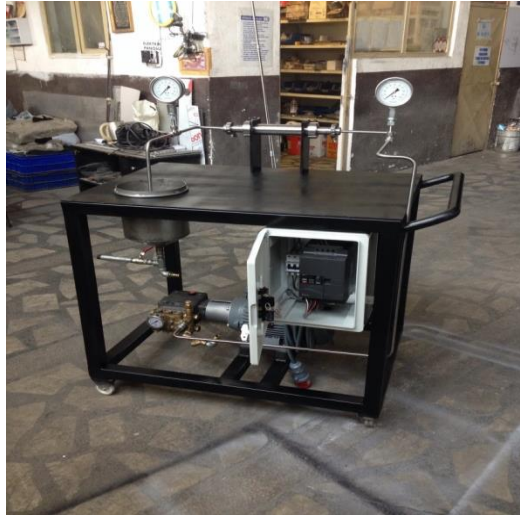
Figure 5.6. The membrane filtration system.
