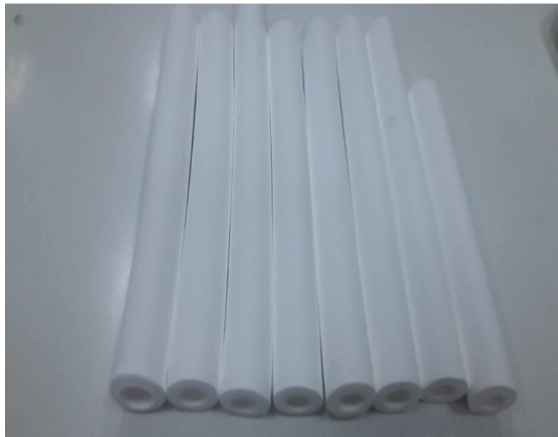
Figure 6.1. Tubular alumina ceramic membrane supports.
