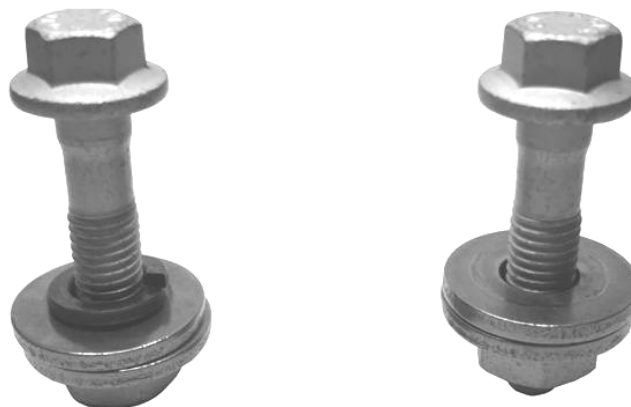
Figure 4.4. Test specimens for ISO-metric thread form with spring washer and new thread form without spring washer, respectively.
