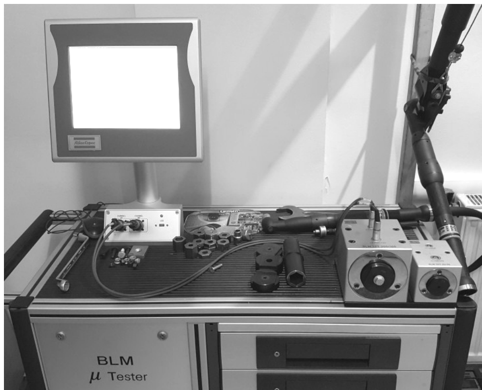
Figure 2.14. Torque-tension test machine in Norm Fastener Co.
