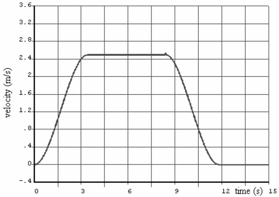
Figure 3.3. The velocity of a point of rope almost contacted to sheave
