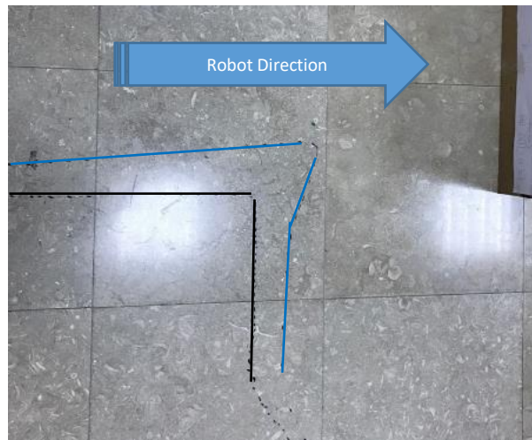
Figure 5.14 Test results of the obstacle avoidance algorithm for mobile robot speeds of 0.5 m/s and 0.8 m/s
