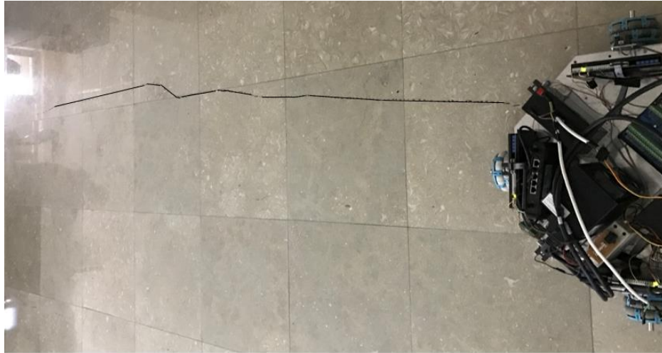
Figure 5.20 Mobile robot's path when 50% performance loss occurs in wheel 2 during the motion in (+) x-direction
