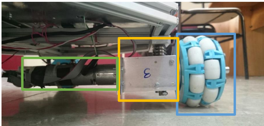
Figure 3.3 Actuation System of the Redundant Mobile Robot
